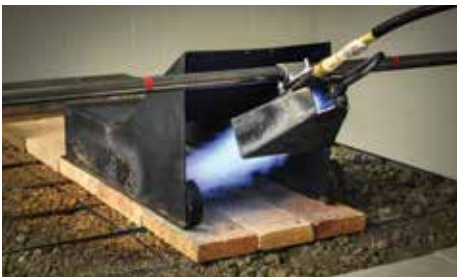
Testing of propane flaming with torch hood
